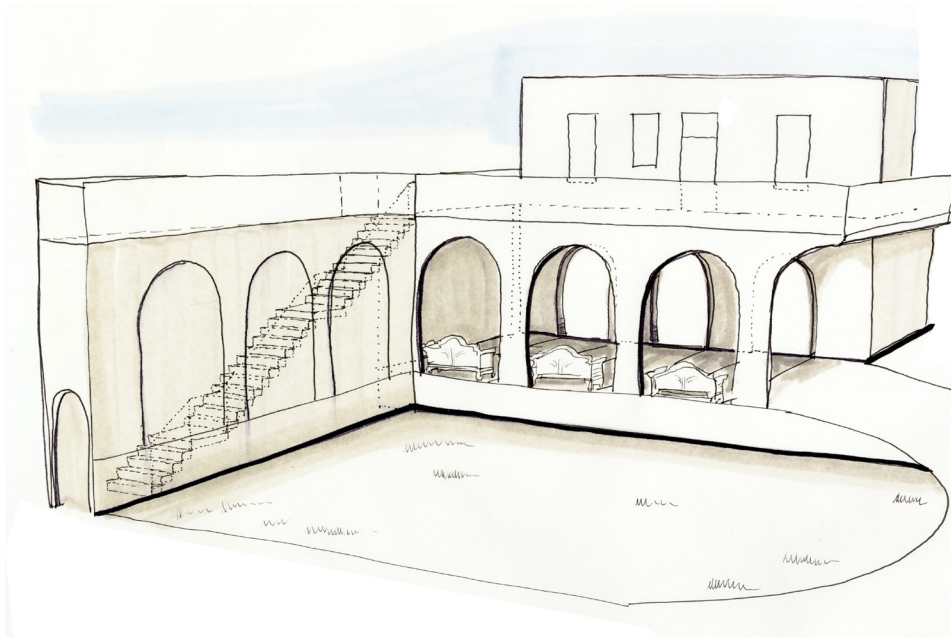
Loggia / Fire Egress: 3rd Floor to 2nd Floor deck c/o a spiral staircase, down to Ground Level via stair behind latticework wall, increases outdoor space by 1,000 sq. ft.
